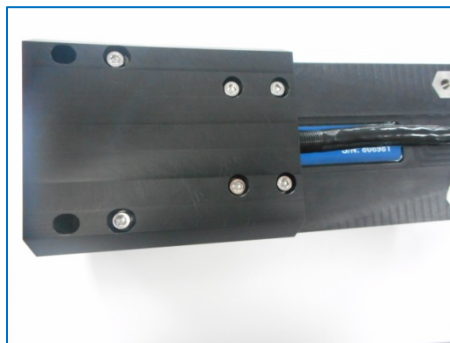
Figure 23: Projector cable clamp in place
