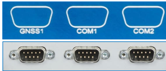
Figure 149: SIMINS Serial Ports
