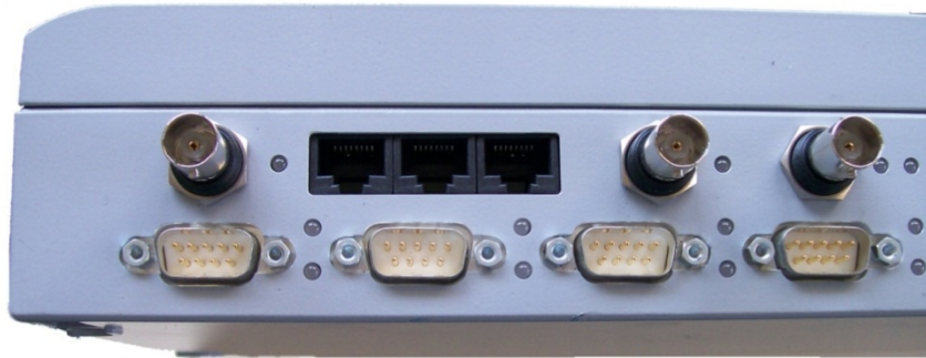
Figure 37: SIM Interfacing Physical Connections
