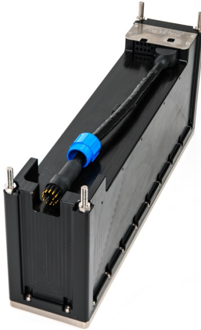
Figure 13: New cable penetrator with a locking ring
