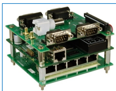
Figure 184: SIM Board Stacks
