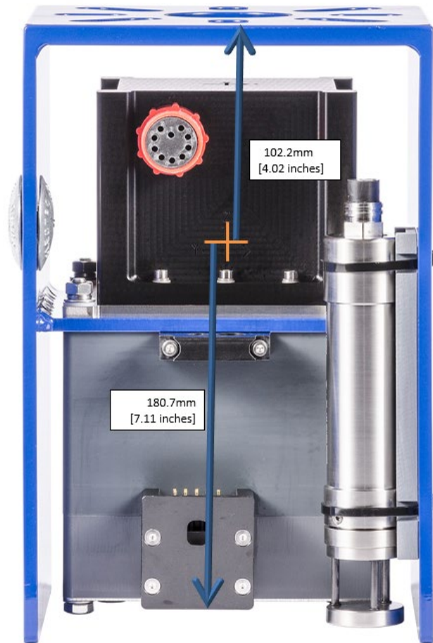
Figure 141: 2020-IMU Vertical Offsets Type 82 IMU
