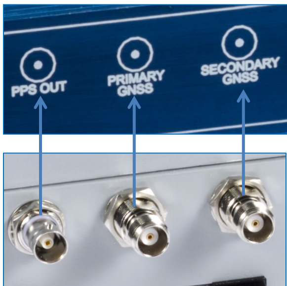
Figure 126: INS BNC & TNC Connections
