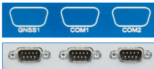
Figure 127: SIMINS Serial Ports
