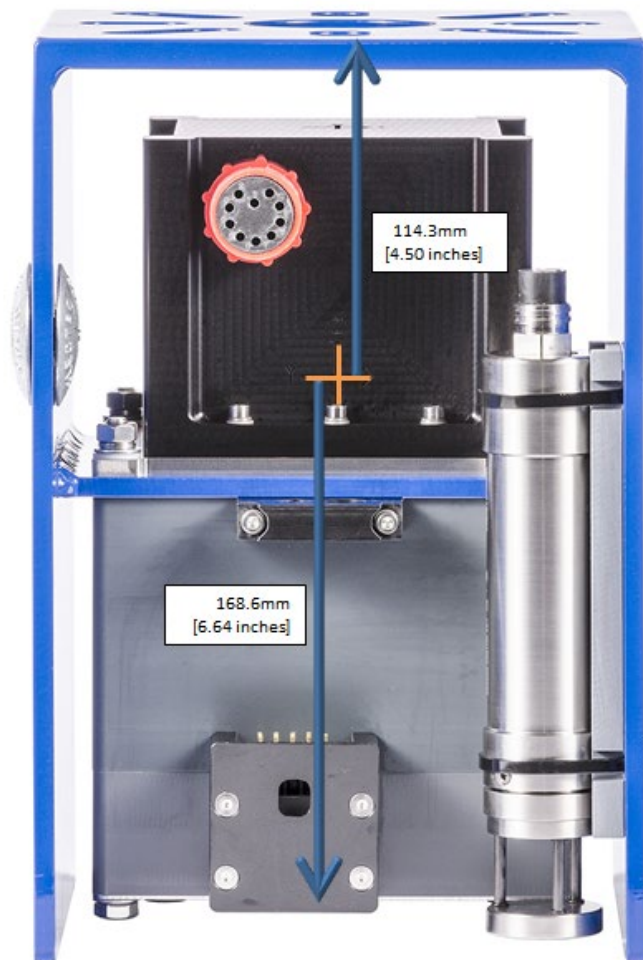
Figure 140: 2020-IMU Vertical Offsets Type 42 IMU
