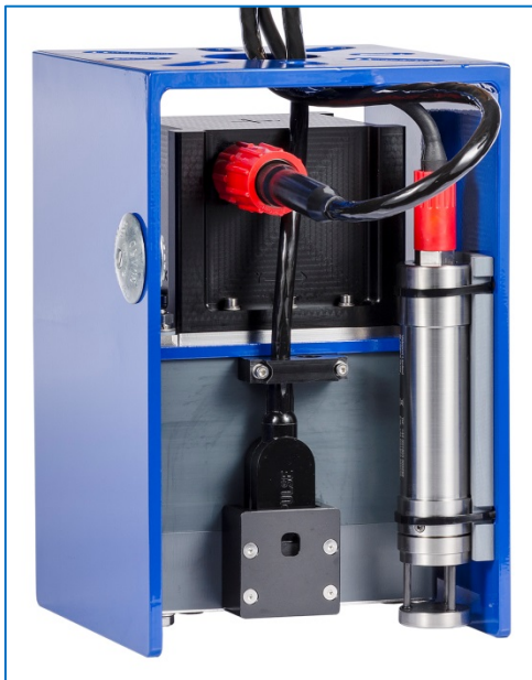
Figure 123: Aft detail of the IMU cable connection
