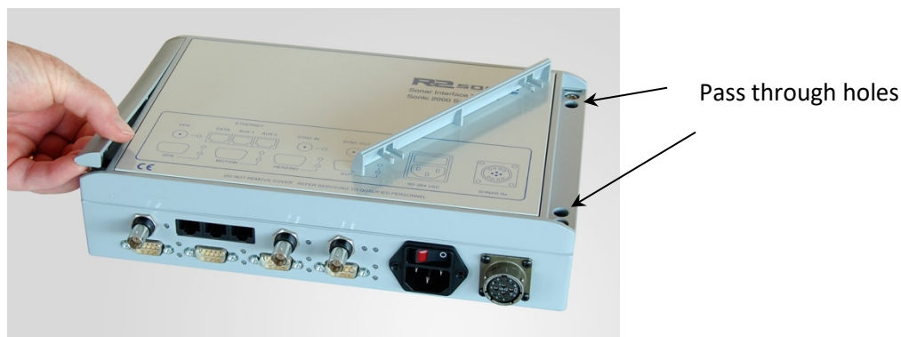
Figure 13: Removal of trim to expose securing holes
