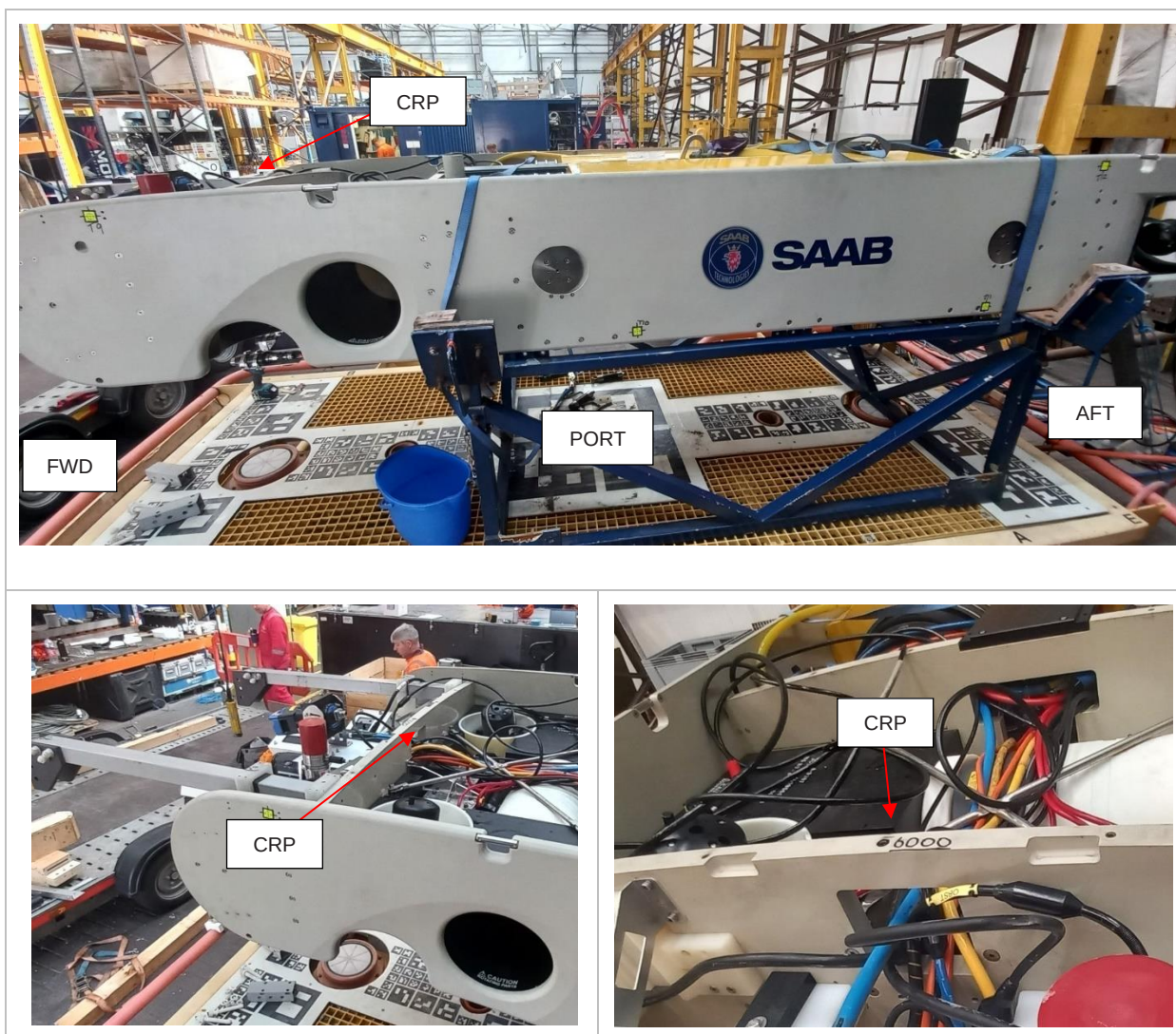
Figure 4: HAUV – CRP Location and Detail
